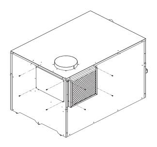
FIG. 4 Metal Panel Covering Side Combustion Air Inlet
